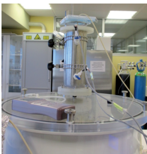
Parts of an experimental equipment for unsaturated column study
